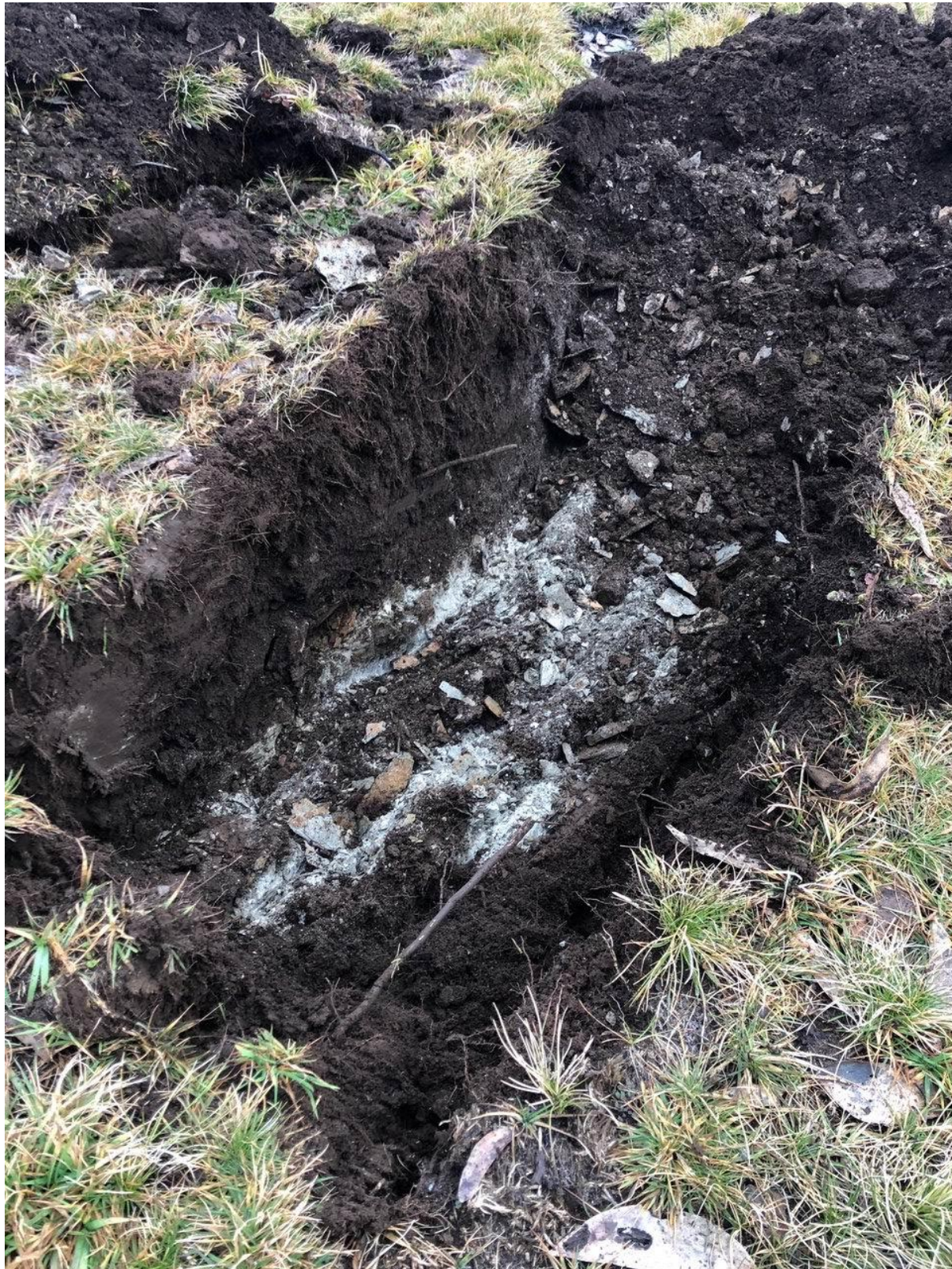
Photo 8 – 10/7/2020 – View of the subsurface profile of test pit 1T, showing topsoil, directly underlain by medium strong slate bedrock.
